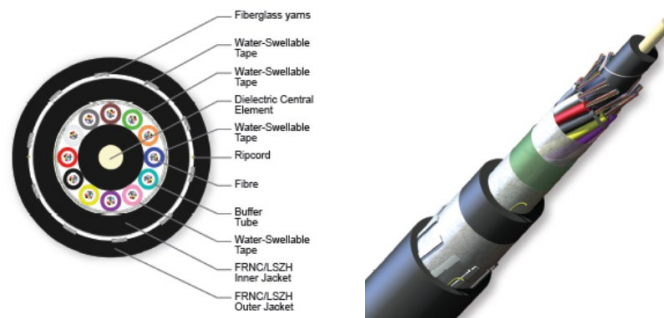
Figure 1. Typical Optical fibre construction
