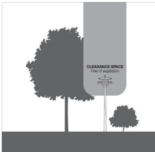
Figure 5 – Uninsulated 66,000-volt electric line in LBRA and uninsulated electric line in HBRA
